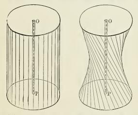
a similar disk at the top. The latter can be turned round on the rod. Vertical threads pass from all points of the circumference of one disk to the corresponding parts of the other, thus forming a cylindrical surface. Then turning the upper disk through any angle less than 180°, the threads will form an hyperboloid of revolution, as shown in the other
